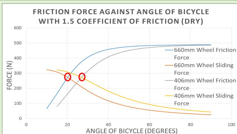
Friction and sliding forces are calculated for different sized wheels. A smaller approach angle reduces the friction force.
