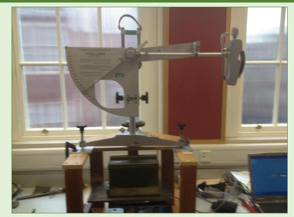
A section of tyre is attached to the end of a pendulum arm. When released, the arm swings down so the tyre can interact with a section of rail.
